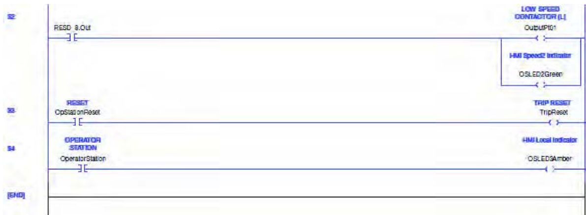
Figure 179 - Two-speed Starter (Operator Station) with Feedback DeviceLogix Program, Part D
