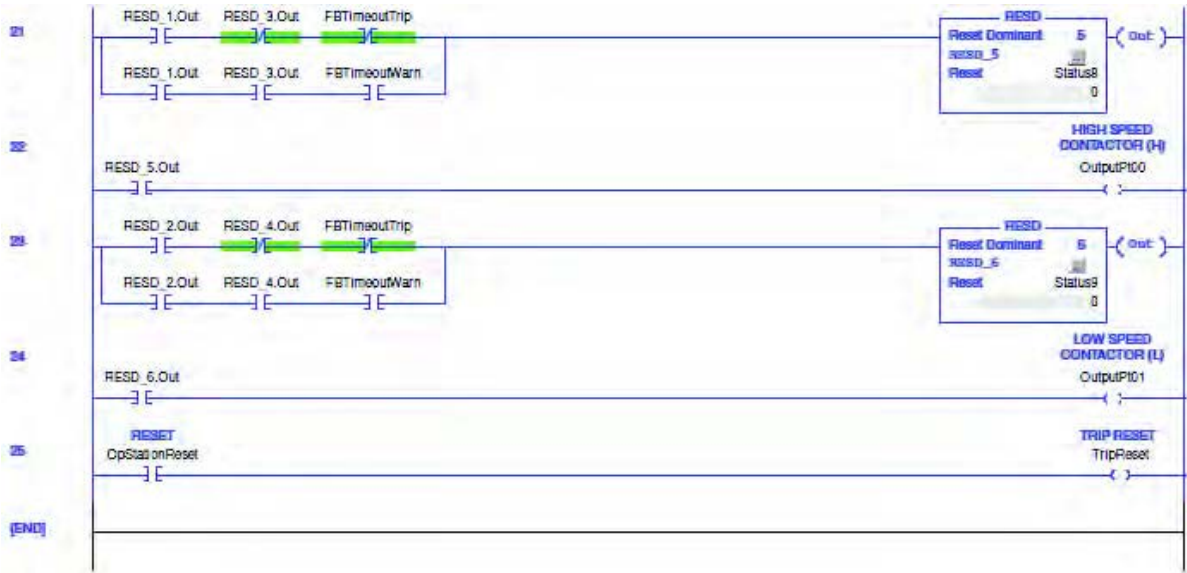
Figure 188 - Two-speed Starter (Local I/O) – Two-wire Control with Feedback DeviceLogix Program, Part C
