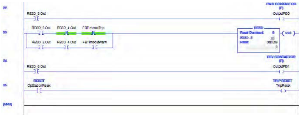
Figure 139 - Reversing Starter (Local I/O) – Two-wire Control with Feedback DeviceLogix Program, Part C
